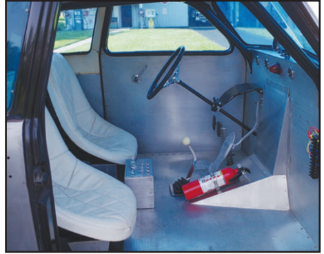
Aluminum fire wall, flooring and door panels, all done to save weight. New electrical panel wired.
