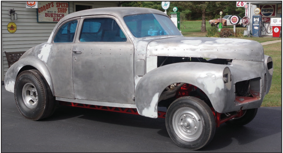
The car in bare metal; outside, under the hood, door jams, and inside truck and fender wells all stripped and sanded.
